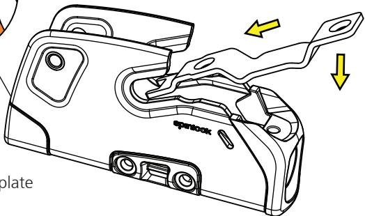
4. Check base plate is correctly aligned
