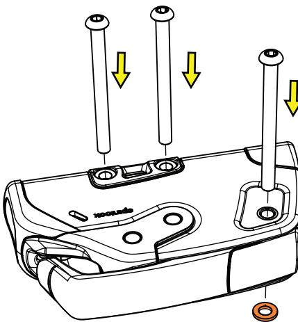
6. Insert fixings - place plastic washer on underside of handle bolt
