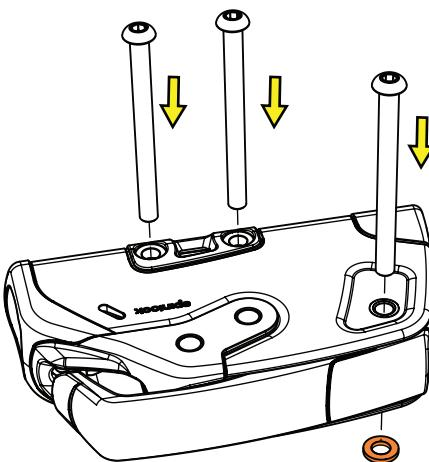
6. Insert fixings - place plastic washer on underside of handle bolt
